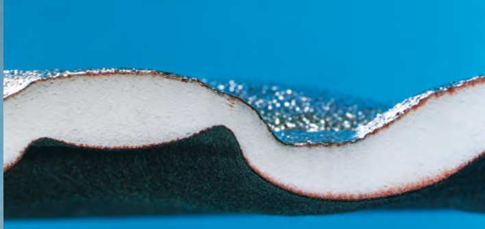
Shaped part with aluminum foil and felt
